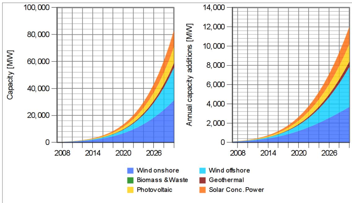
Figure 89: Development of renewable electricity generating capacity in the Middle East ("Low Variant") [EWG; 2008].
