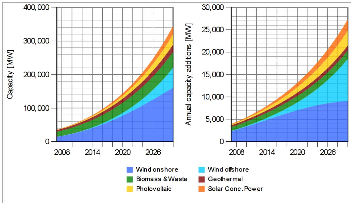
Figure 65: Development of renewable electricity generating capacity in OECD North America ("Low Variant") [EWG; 2008].
