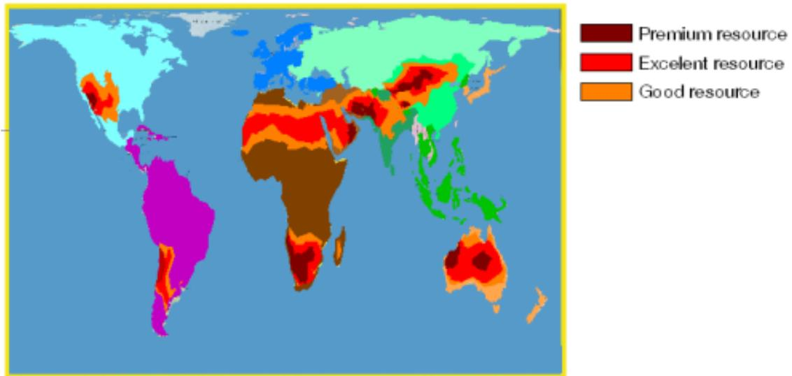
*Figure 92: Solar thermal Power resources mapped to the “Peters projection” (showing true surface area), disaggregated into the regions used by the IEA [EWG; 2007].*
