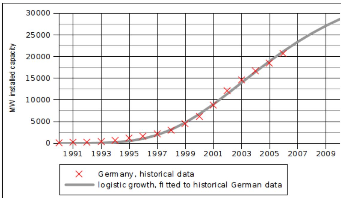
Figure 8: Example of fitting the logistic growth function used in the “REO 2030” scenarios to historical data of Wind Energy development in Germany.
