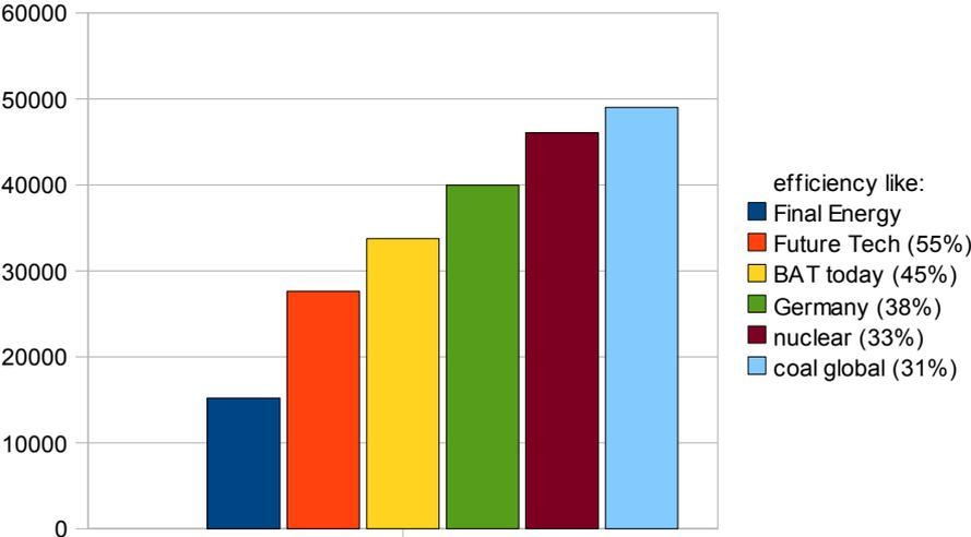
Figure 28: Converting electricity from renewable technologies into primary energy, different assumptions off plant efficiencies. [EWG; 2008]
